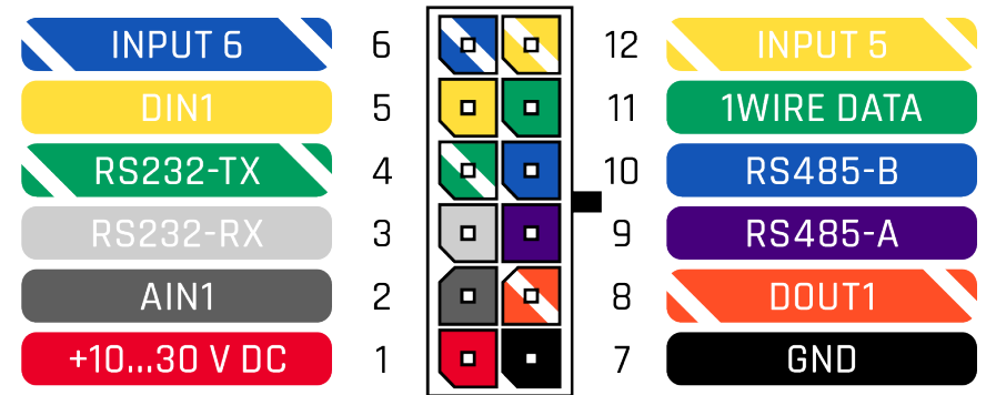
Figure 2 FMB125 2x6 socket pinout
